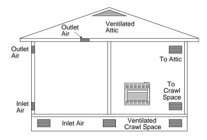
Figure 9 - Ventilation Air from Outdoors
